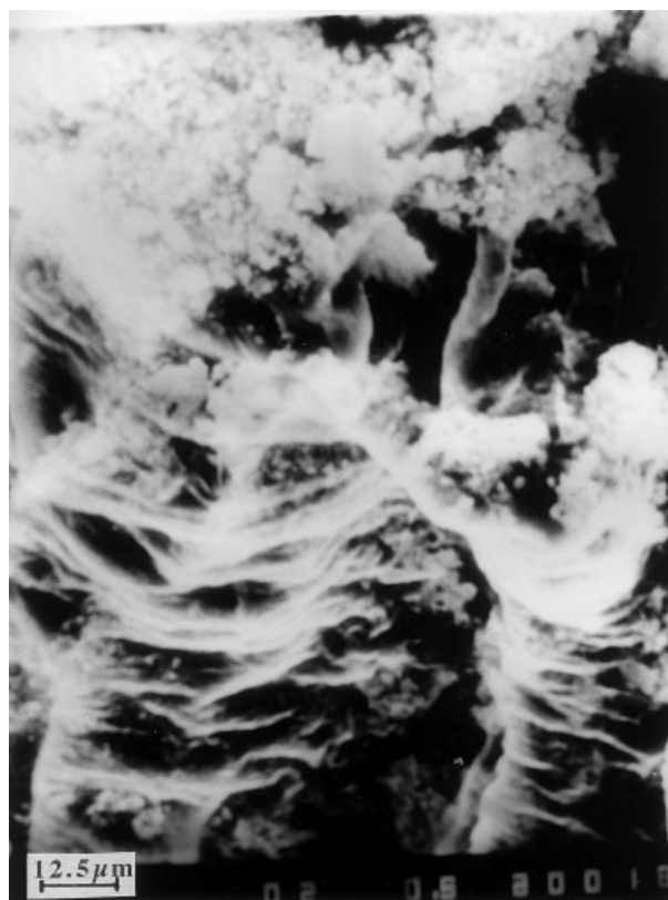
Figure 12 SEM micrograph of PFu/P2ClAn (magnification 800X, bar = 12.5 μm).
