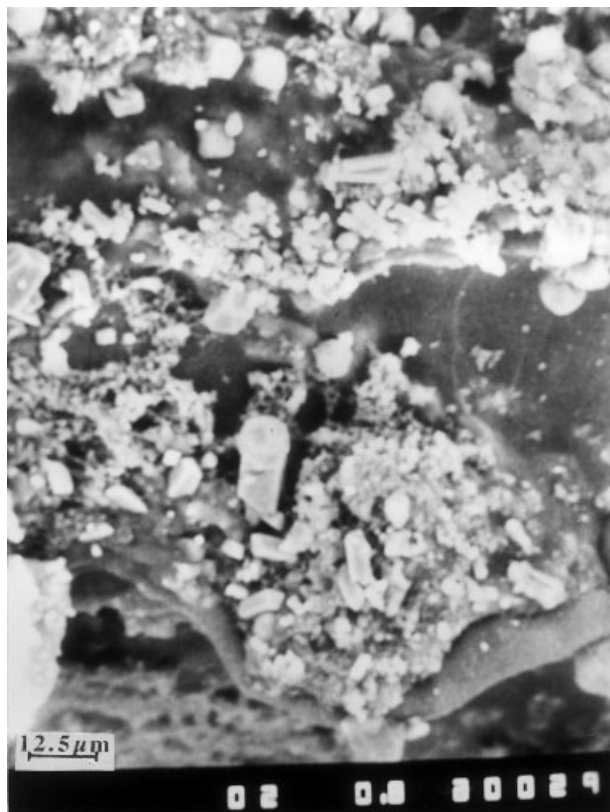
Figure 11 SEM micrograph of PFu (magnification 800X, bar = 12.5 μm).
